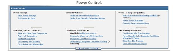
From here, you have easy access to the *Wake-on-LAN* Wizard, which allows you to "wake" computers. There are also instructions on how to set up right click Wake-on-LAN. With this feature enabled, you can right-click on any computer listed in the BigFix *Computers* tab and select it for Wake-on-LAN. The right-click Wake-on-LAN feature will only work if you are in the same subnet as the BigFix Clients or if your network allows you to send UDP packets to the broadcast address of different subnets.
