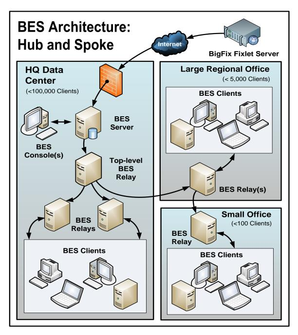
Often these locations are configured in a hub-and-spoke arrangement. This scenario builds on the previous one, but the hub-and-spoke configuration permits more levels in the BES Relay hierarchy.
