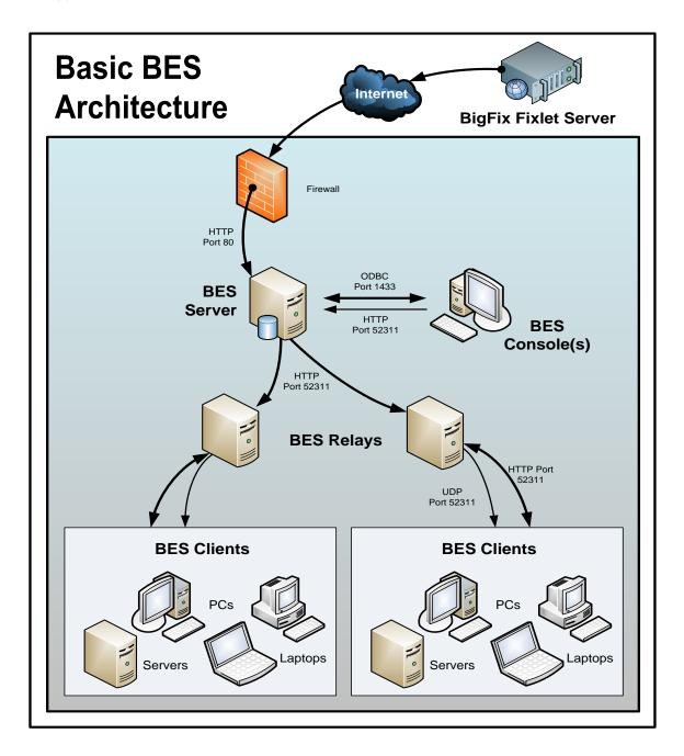
The BES Consoles oversee all this activity. They connect to the BES Server(s) and periodically update their displays to reflect changes or new knowledge about your network. The BES Console operator can then target actions to the appropriate computers to fix vulnerabilities, apply configuration policies, deploy software, etc. The progress of the actions can be followed in near real-time as they spread to all the relevant computers and, one by one, address these critical issues.
